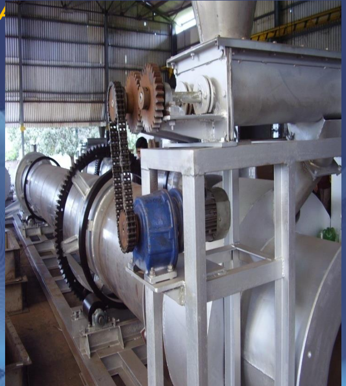
DIRECT FIRED ROTARY CALCINER
