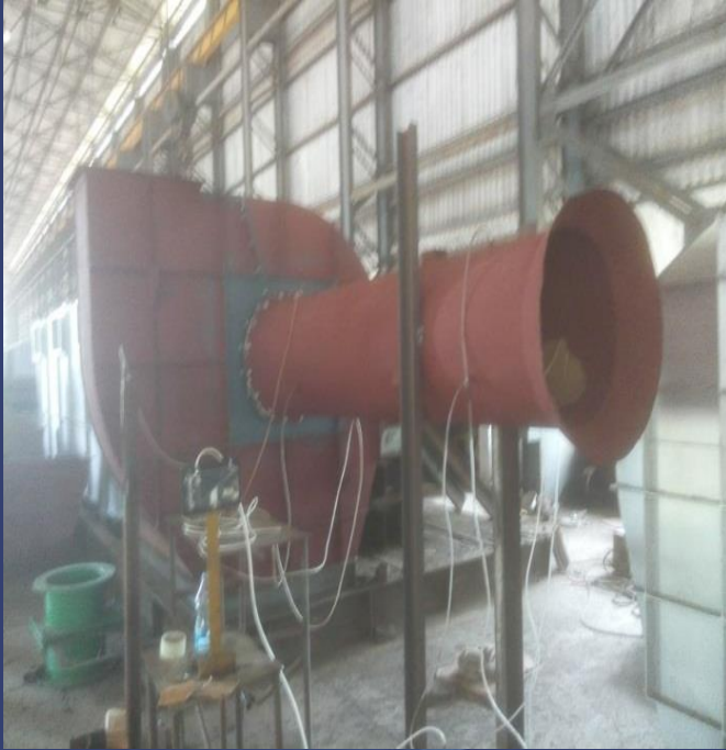
PERFORMANCE TESTING OF FANS
